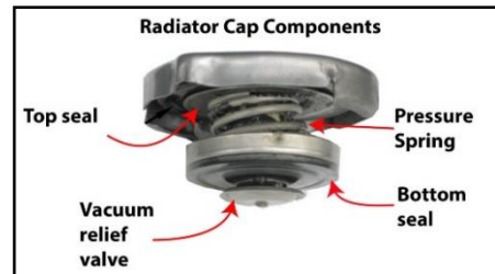
Figure 2. Functional parts of a radiator cap.
