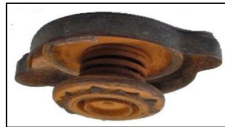
Figure 3. A rusty radiator cap.
